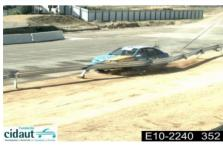
**Test**: TB32 (car 1.500 Kg., 110 Km/h, 20°)
