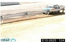
Test: TB11 (car 900 Kg., 100 Km/h, 20°)
