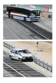
**Test:** TB51 (heavy vehicle 1.500 Kg., 110 Km/h, 20<sup>o</sup>) **Code:** 448 **Date:** 27/09/2007 **Laboratory:** AISICO (Italy)
