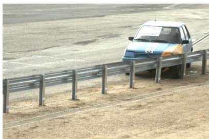
Test: TB11 (car 900 Kg., 100 Km/h., 20°)
